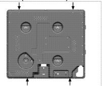
Place the burner plates, burner plate caps and grills back to their seating after installation.
