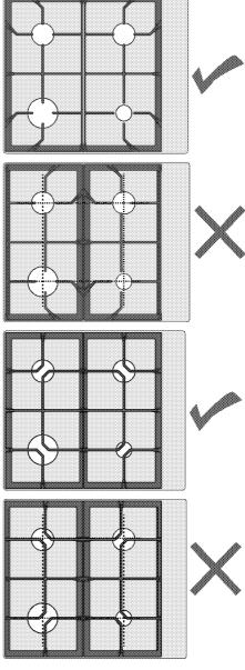
**Assembling the burner parts** Place the parts as in the figure after cleaning the burners.
