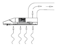
Your cooker hood can be configured to operate in the ducted or re-circulating mode
