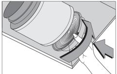
Remove aluminium grease filter.
