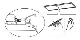
Make the electrical connections of the appliance. Your appliance uses 2X2 W spot LED lamp. For replacing the lamps, push downwards on the holder from its behind, turn it counter-clockwise, and
