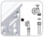
There is a filter at the end of each water intake valve at the rear of the machine and also at the end of each water intake hose where they are connected to the tap. These filters prevent foreign substances and dirt in the water to enter the washing machine. Filters should be cleaned if they are dirty.
