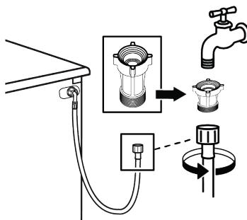
**EN:** According to the relevant EN 61770 / DIN standards, the appliance must be connected to a water supply system with a check valve, service spare part number 2860940100/C00846477 or equivalent.
