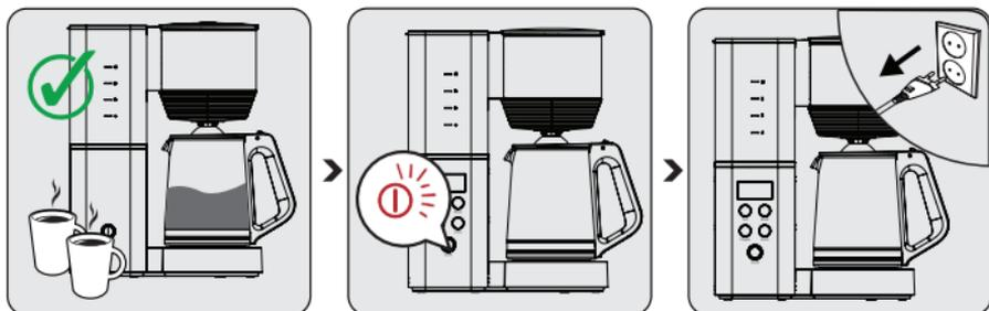
To serve, remove the glass carafe once the brewing is complete (about one minute after the coffee has finished dripping).
