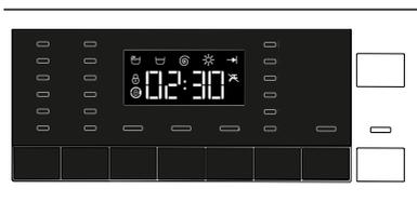
There is a locking system on the loading door of the machine that prevents opening of the loading door in cases when the water level is unsuitable for door opening. "Loading door locked" light in the panel turns on when the loading door is locked.
