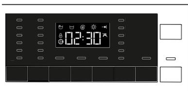
The programme is cancelled when the machine is turned off and on again. Press and hold **On / Off** button for 3 seconds. After the countdown as "3-2-1" on the display is over, the machine turns off.
