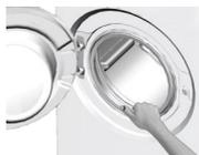
After every washing and drying make sure that no foreign substance is left in the drum. If the holes on the bellow shown in the figure are blocked, open the holes using a toothpick.
