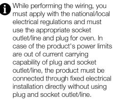
1. If it is not possible to disconnect all poles in the supply power, a disconnection unit with at least 3 mm contact clearance (fuses, line safety switches, contactors) must be connected and all the poles of this disconnection unit must be adjacent
