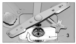
Press the two pawls on the coarse filter inwards and separate the coarse filter from the assembly.
