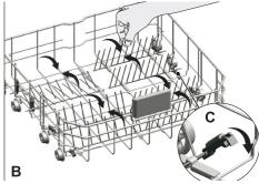
Bringing the tines to the horizontal position by holding them from the tips may cause them to bend. Therefore, it will be appropriate to bring the tines in the middle to horizontal or vertical position by holding them from their stems and pushing in the direction of arrow.
