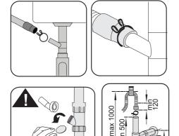
Drain pipe must be connected to the sewage system and it should not be connected to any surface water.
