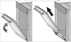
4. Remove the front door by pulling it upwards to release it from the right and left hinges.
