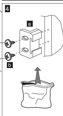
**Note:** Installation step for 2, screws for connecting top plastic part should not be screwed very hard, because of moving the plastic part easily left or right side.
