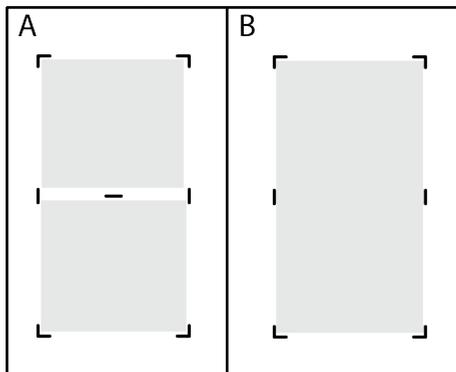
When the two separate cooking zones (shown in the figure A) are combined as a wide surface cooking zone shown in the figure B, the separating light should go off. When the wide surface cooking zone is returned back into two separate cooking zones, the separating light should be illuminated.
