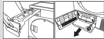
2. Drain the water in the tank.
