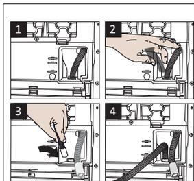
1-2 Pull hose at the behind of the dryer by hand in order to disconnect it from where it is connected. Do not use any tools to remove the hose.
