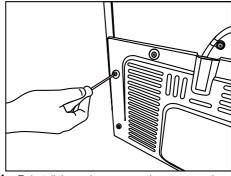
To install the wedges, remove the screws on the product and use the screws supplied together with the wedges.
