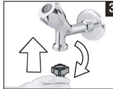
3 Open the taps completely after making the hose connection to check for water leaks at the connection points.
