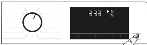
Press the **Start/Pause** button to switch the machine to pause mode.
