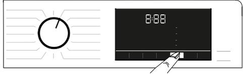
When you select a new washing programme, press the Auxiliary Function Selection button to set the drying option suitable for this programme.
