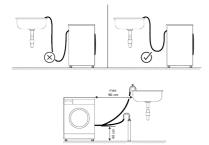
b. Connect the hose to a minimum height of 40 cm and a maximum height of 90 cm.
