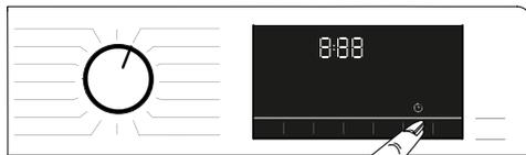
In order for the End Time function is activated and the programme is completed at the end of the specified time, you must press **Start/Pause** button after adjusting the time.
