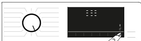
When the Remote Control is on, you can only manage, turn-off and status follow-up operations through your washing machine. And all functions except child lock can be managed through the application.
