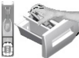
Clean the detergent drawer at regular intervals (once every 4 to 5 wash) as mentioned below to prevent accumulation of powder detergent. Clean the syphon if excess amounts of water and fabric softener mixture remains in the softener compartment.
