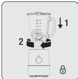
Place the glass container (3) to motor unit (6) upright, turn it to the "8" symbol to lock it in its place.
