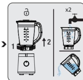
Remove the jug (3) from the motor unit (6). Rinse with water to clean up large food residues that can pile up in the container.
