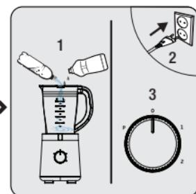
Place the jug (3) in its place. Add warm water and 1 to 1 ½ unit of liquid detergent and operate the blender in high speed for a few seconds.
