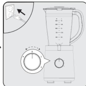
Plug the appliance to the socket and start operating by selecting the speed level (7).
