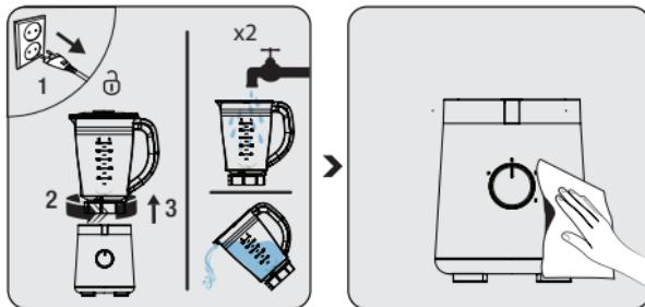
Unplug the appliance. Remove the jug (3) from the motor unit (6) and rinse it with water. If necessary, repeat the same steps.
