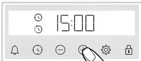
» After the cooking end time is set, the ⌚ symbol and the ⌚ symbol with the time period symbol will appear constantly on the display. As soon as cooking starts, the ⌚ symbol disappears.
