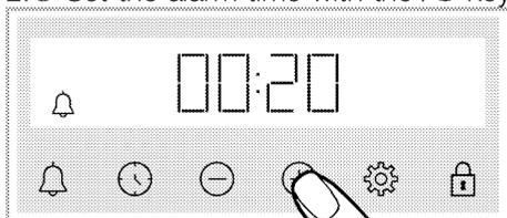
» After setting the alarm time, the
