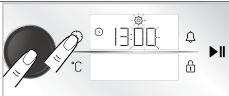
4. Set the minute by turning the oven control knob to right/left. Approve the setting by pushing the oven control knob once or touching the ⌚ key once.
