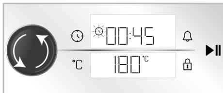
**i** The baking time increases by 1 minute in the first 15 minutes and by 5 minutes after 15 minutes.
