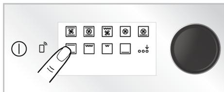
3. If the function you want to activate is not among the operating functions that appear first on the function display, you can activate the operating functions in the lower row by touching "Extra function activation"
