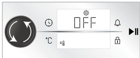
3. Activate the quick preheat (Booster) setting by touching the ⌚ key or pushing the oven control knob once.
