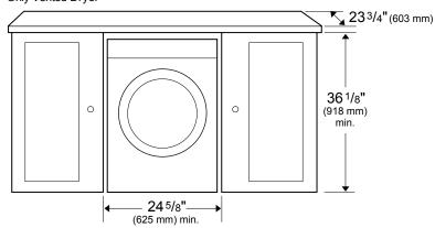
Required Minimum Clearances: (Stand Alone, Side by Side, or Stacked)
