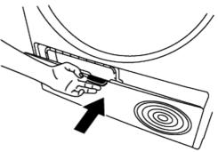
Sharp Edges - To reduce the risk of injury, use care when cleaning the condenser or evaporator coil fins. You can clean by hand, provided you wear protective gloves. Do not try to clean with bare hands. The condenser fins may damage your hands. Cleaning from left to right may damage the condenser fins. This may lead to drying issues.
