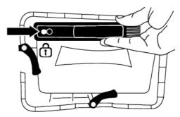
After the cleaning process is completed, place the air deflector cover to its place, move the latches to close it and close the toe board.
