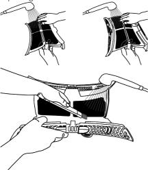
Insert the fibre filters on one another and place it back in its place.
