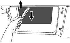
After cleaning the filter, door and the condenser, drag the brush to the right and lock it in its place.
