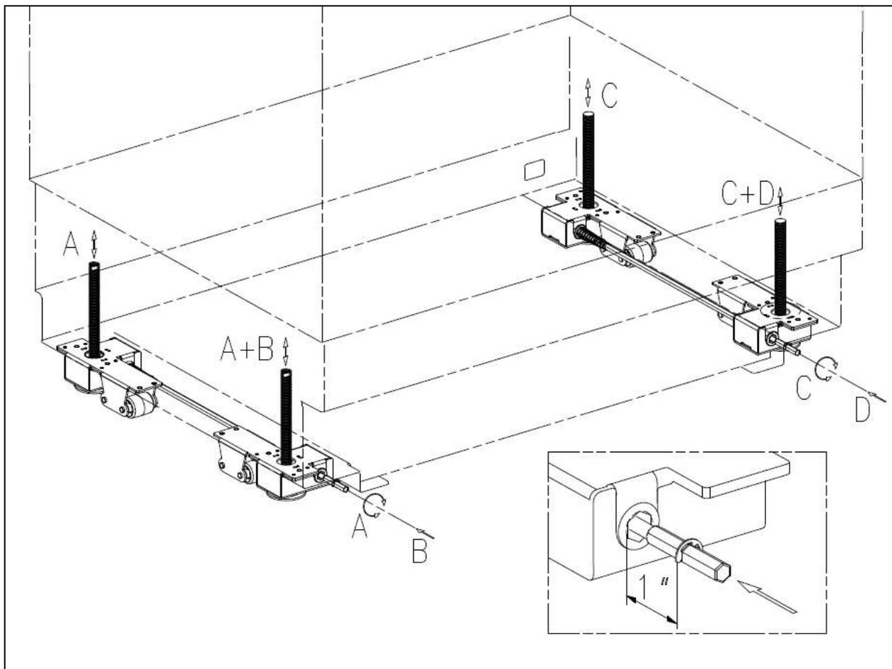
**A+B** – The Front Left section will rise if you push the left adjustment rod forward by 1" and rotate it clockwise
