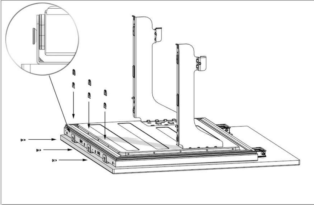
A total of 3 mm washers must be placed on the FRZ Door (2+1) on the condition that all furniture dimensions are suitable. Washers to be used are determined based on the kitchen design.
