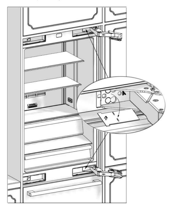
• Remove the lower right hinge by loosening its 2 screws and fix it to its slot at the upper Left side.
