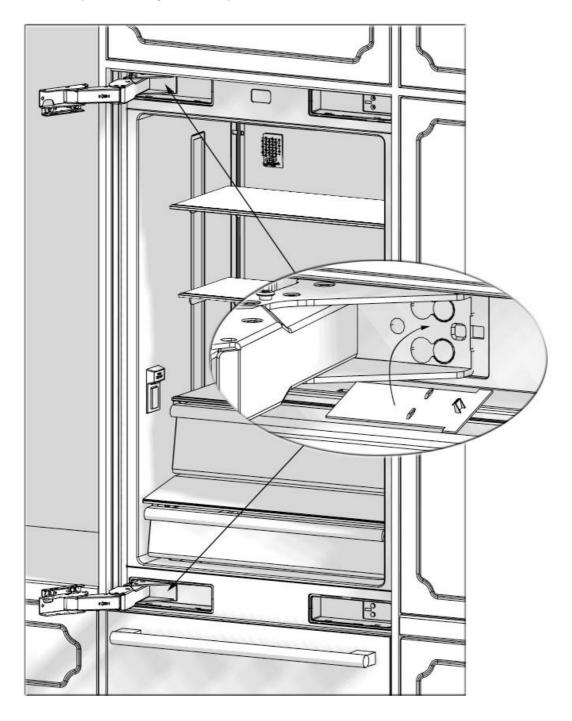
• Attach the Hinge Slot Caps removed from the left side to the Hinge Caps at the right side.
