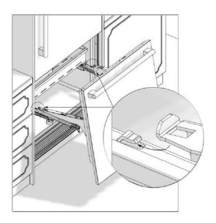
• Fix the Freezer Furniture door assembly onto the rails with 2 screws.
