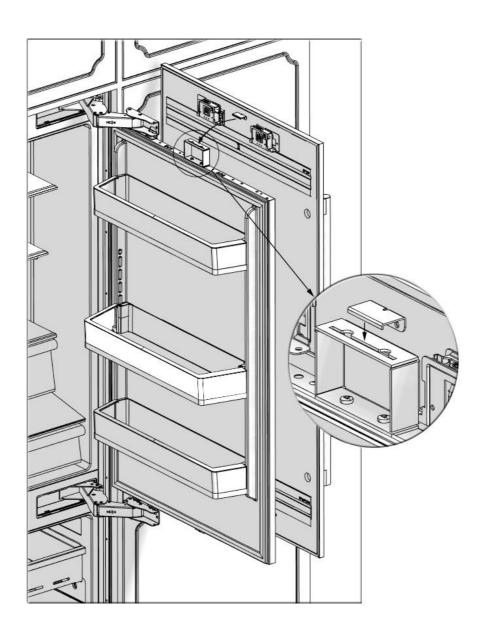
• Group the FF Upper Mechanism with 4 screws.
