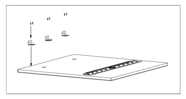
• Attach the 3D adjusting mechanisms you have removed from the door to the door cradles.
