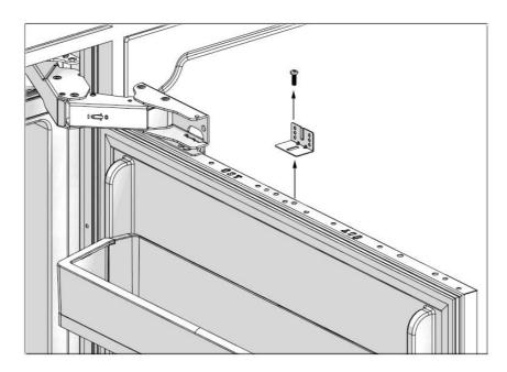
• Attach the FF Hanger Bracket (13) part in the mounting box to its place with the help of 2 screws (16).
