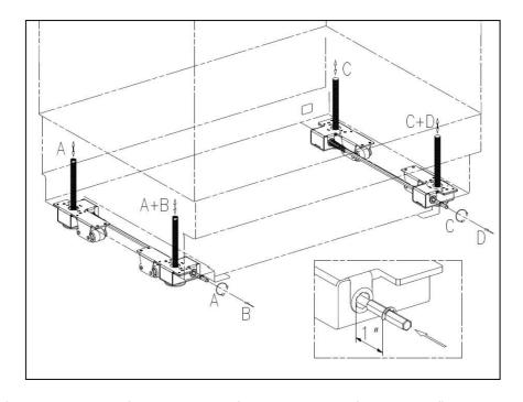
A+B – The Front Left section will rise if you push the left adjustment rod forward by 1" and rotate it clockwise
