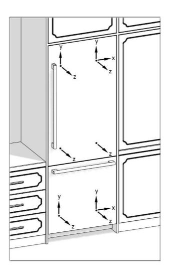
• After completing door adjustments, attach the brackets to the middle section of the Fridge door.
