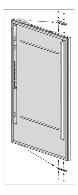
• Attach the Hanger Sheet (13) using 2 screws (16).
