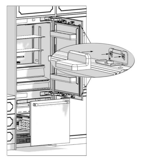
• Tighten the screws together with enough Crescent Washers to cover the clearance under the upper brackets of the Freezer Door.
