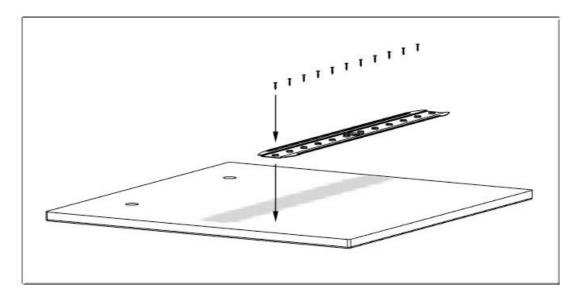
• Attach 3 sheet metal brackets (25) using 2 screws (26) for each.
