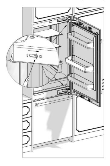
Remove 4 Fixing Brackets on the fridge door.
