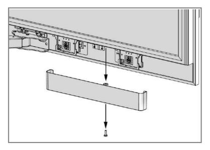
Remove FF Lower and Upper Bracket screws.
