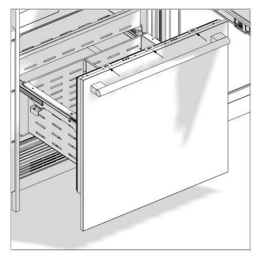
• Remove 3 Fixing Brackets at the lower section of the freezer door.
