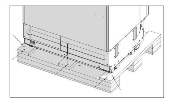
• Hold the refrigerator firmly, put its weight to the front and push the Wooden Pallet's rear part (from which you have removed the screws) sideways to remove it.
