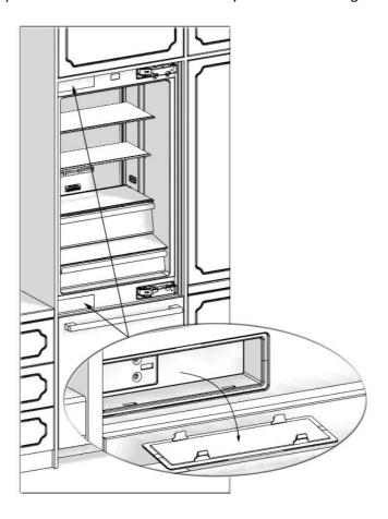
• Remove the Screw caps of the hinges.
