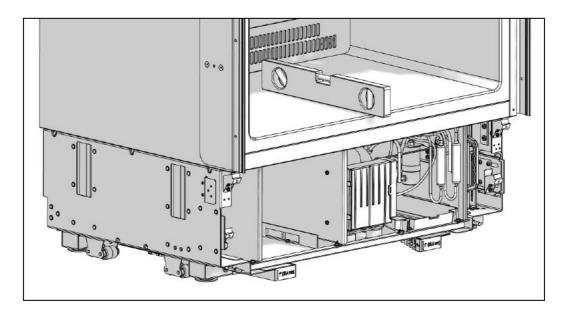
After adjusting the adjustable feet, check the flatness in both width and depth directions.
