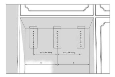
• Use a drill to create holes for Dowels (8) at the marked points.  $(5/16" - \emptyset8)$
