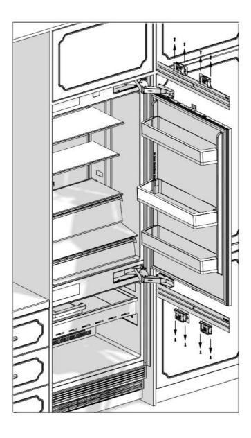
Remove the 3D Adjusting Mechanism Assembly from the lower part of the FRZ PU Door.
