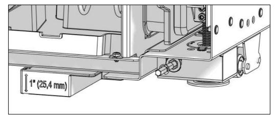
• The rear feet are adjusted via Bubble Level Tool.
