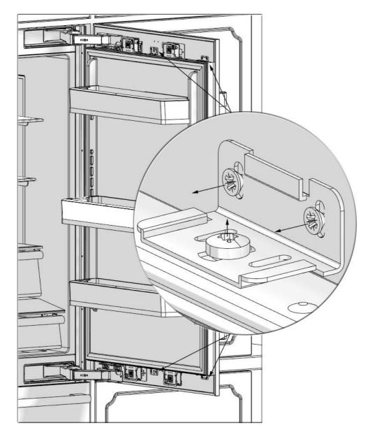
Remove the screw of FF Upper and Lower mechanisms.
