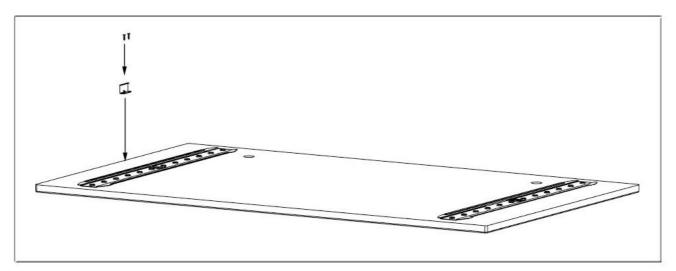
• Attach the 3D adjusting mechanisms you have removed from the door to the door cradles.
