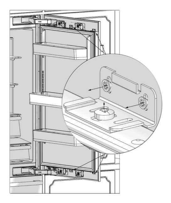
• Loosen 3 bracket screws at the upper section of the freezer door.
