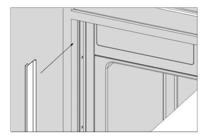
• Attach the upper closing part (4) onto the upper connection bracket.
