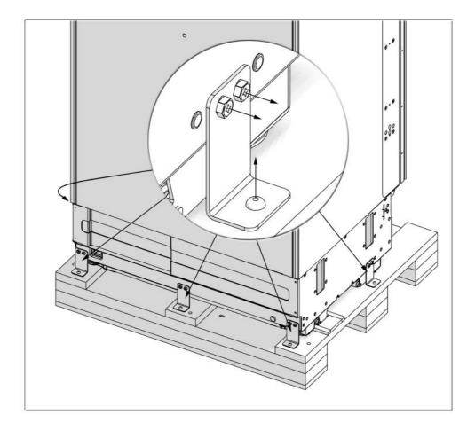
• ove the screws that hold the rear foot of the Wooden Pallet.
