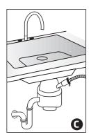
• The maximum length must not exceed "approx. 13 feet" (4000mm). Otherwise, the cleaning process is negatively influenced.
