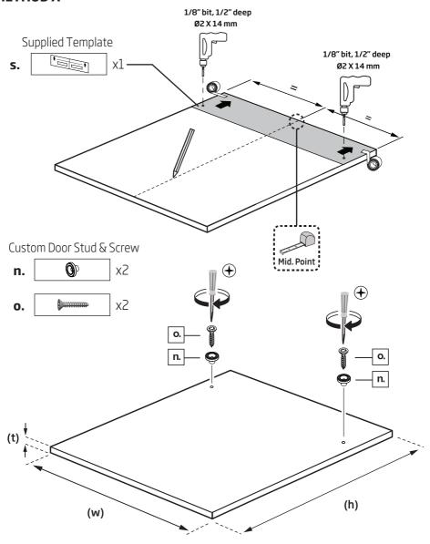
**Height (h):** 27  $^9/_{16}$  " to 29  $^{15}/_{16}$ " (700 mm - 760 mm) Tall Tub Models Only **Height (h):** 26 " to 28  $^{11}/_{32}$ " (660 mm - 720 mm) Standard Tub Models Only
