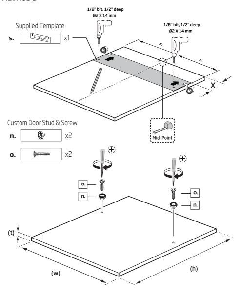
**Height (h):**  $27^9/_{16}$  " to  $29^{15}/_{16}$ " (700 mm - 760 mm) Tall Tub Models Only **Height (h):** 26 " to  $28^{11}/_{32}$ " (660 mm - 720 mm) Standard Tub Models Only
