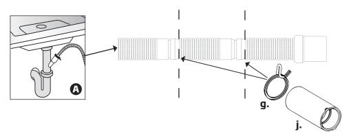
Due to the local building code requirements, some dishwasher installations require hooking up. Since the connection diameter is different than standard discharge hose connections, please use the connector piece provided with the machine with instructions illustrated.
