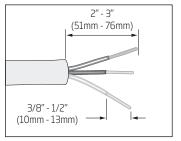
Electrical supply cords must be a minimum #14AWG copper wire. The dishwasher is designed for an electrical supply of 120 V, 60 Hz, AC, connected to a dedicated, properly grounded electrical circuit with a fuse or breaker rated for 15 amperes.
