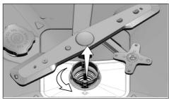
2. Pull out the metal / plastic filter (3) from the seating.
