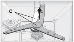
To remove and clean the lower impeller assembly together, hold by one hand from the (C) points shown in the figure and pull up to remove. After cleaning, follow these steps in reverse order to reinstall the impeller assembly.
