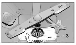
3. Press the two tabs on the coarse filter inwards and separate the coarse filter from the assembly.
