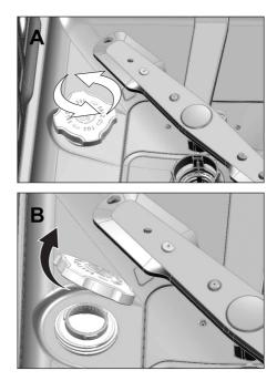
Add 4 cups of water to salt reservoir of З. your machine only in initial use (C).
