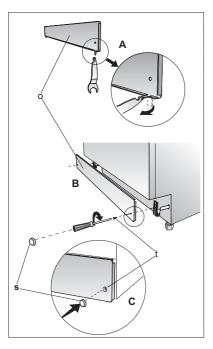
Lock the toe kick brackets as shown with the plastic tab in the figure C by pushing the plastic tab on the dishwasher into the teeth of the bracket  $(\mathbf{C})$ .
