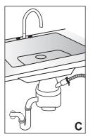
Every disposal has a hook up for a dishwasher; consult your disposer manual for correct connection. (Figure **C**)
