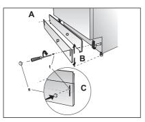
If the enclosure height is above  $33^1/16''$  (840mm) use "o" and "p" labelled toe kicks together. Make sure the slotted toe kick "p" is on the outside so you can adjust height of the toe kick. Installation should be done following the steps illustrated in the figures A, B and C respectively.
