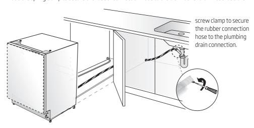
Note that the marks on the rubber connection hose should be on the drain hose side
