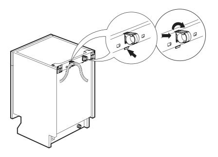
Now place the dishwasher into the opening and get ready to connect all hoses and electrical connections.
