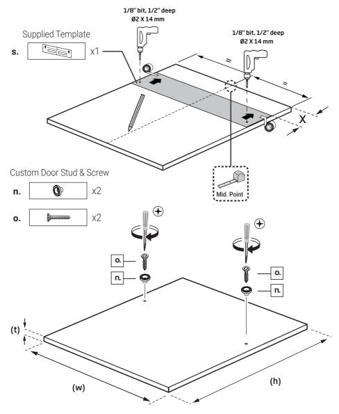
Height (h) : 26 " to 28 <sup>11</sup>/<sub>32</sub> " (660 mm - 720 mm) Width (w) : 17 <sup>3</sup>/<sup>s</sup> " to 17 <sup>5</sup>/<sup>s</sup> " (442 mm - 448 mm) Thickness (t) : Min. <sup>11</sup>/<sub>16</sub> " (18 mm) Weight : 5.5 lbs to 12.1 lbs (2.5 kg - 5.5 kg)
