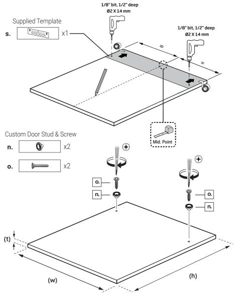
Height (h) : 26 " to 28 <sup>11</sup>/<sub>32</sub> " (660 mm - 720 mm) Width (w) : 17 <sup>3</sup>/<sup>s</sup> " to 17 <sup>5</sup>/<sup>s</sup> " (442 mm - 448 mm) Thickness (t) : Min. <sup>11</sup>/<sub>16</sub> " (18 mm) Weight : 5.5 lbs to 12.1 lbs (2.5 kg - 5.5 kg)
