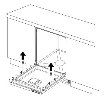
Secure the custom panel to the product through hole 5 with the one in 5/8 inch (Ø 4mm x 42mm) supplied screws on each side.
