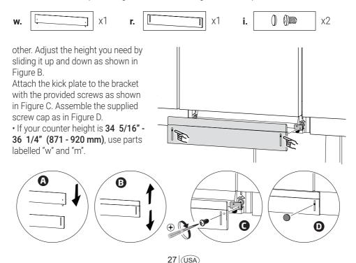
Attach the "w" and "m" pieces together as shown in Figure A. These parts can slide into each other. Adjust the height you need by sliding it up and down as shown in Figure B.
