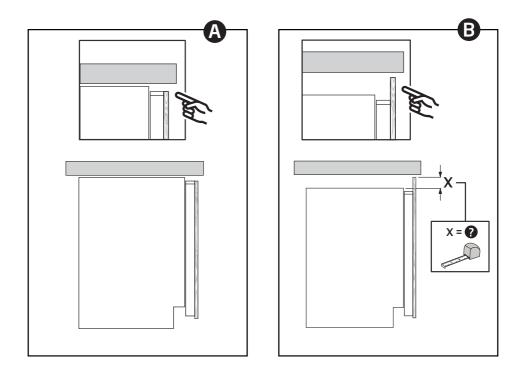
If the custom panel flush with the top of the display as shown in Figure A, place the template as in Method A.
