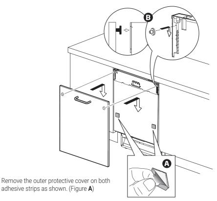
Take the panel and slide the mounting studs into the channels on each side of the door as shown. Slide the panel down to place it. (Figure  $\mathbf{B}$ )
