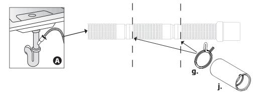
Due to the local building code requirements, some dishwasher installations require hooking up. Since the connection diameter is different than standard discharge hose connections, please use the connector piece provided with the machine with instructions illustrated.
