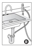
The maximum length must not exceed "approx. 13 feet" (4000mm). Otherwise, the cleaning process is negatively influenced.
