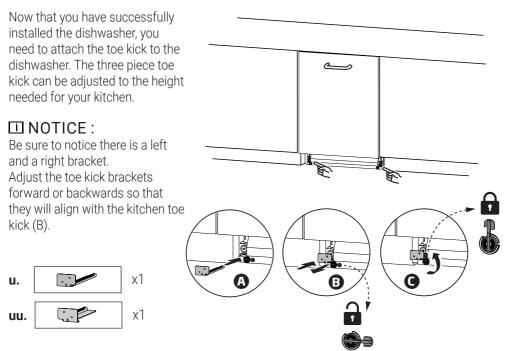
Place parts labelled "u" (left) and "uu" (right) to the channel shown in Figure A for both sides as shown in Figure B. Then fix them in the direction shown with the arrow in Figure C.
